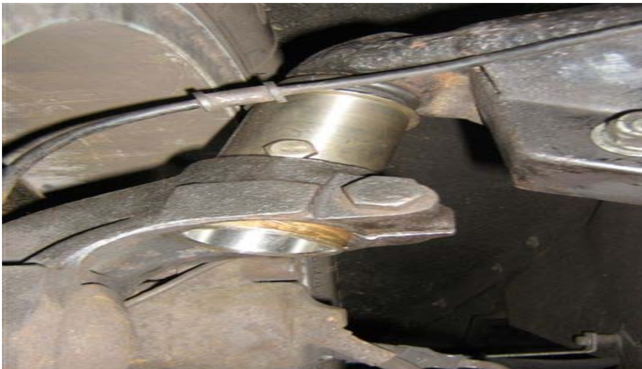
PHOTO 2 New collar fitted
