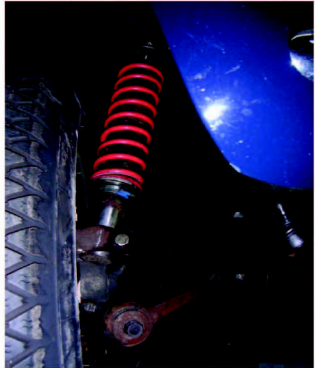
Evaluation of the basic design parameters using a rough-and-ready strut made from several parts found in my workshop
